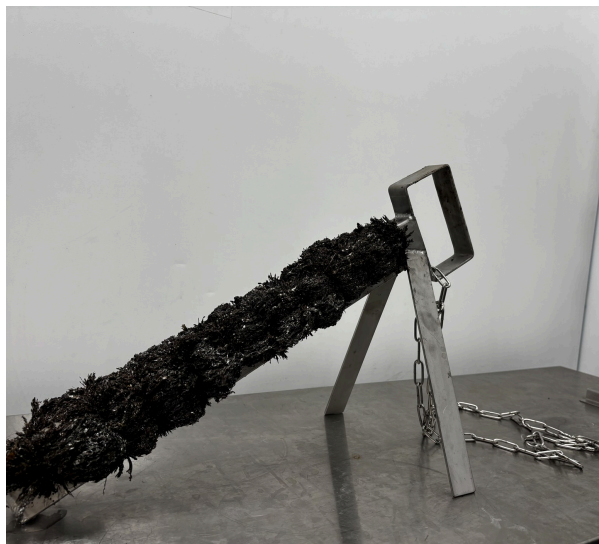
Open-body Ditch Magnet loaded with dry swarf in our workshop. The magnets hold along the full length of the body.
