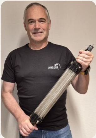
XWW 35 E-Line String Magnet, 3½" OD. Designed and manufactured by Innovar.
