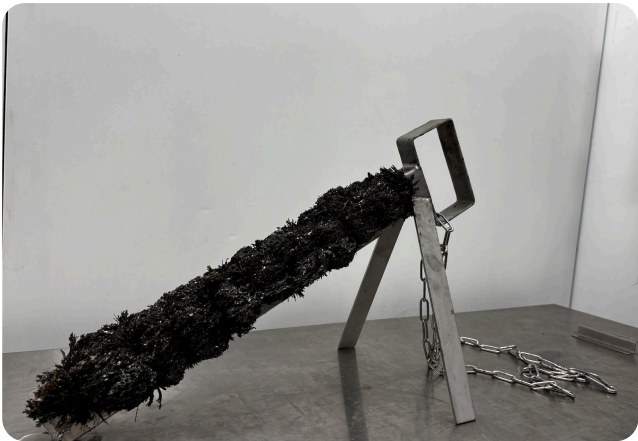
Open-body Ditch Magnet loaded with dry swarf in our workshop. The magnets hold along the full length of the body.
