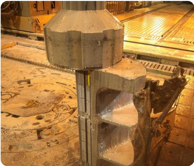
The insert carrier on the 12" Fishing Magnet at the rig floor. Recovered to surface on the second run.
